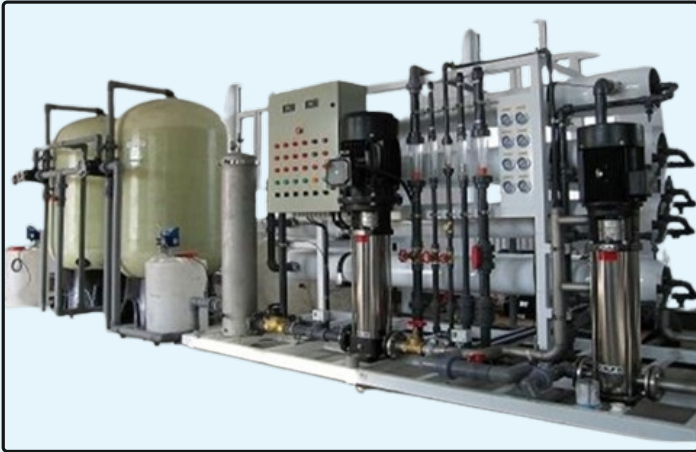
REVERSE OSMOSIS SYSTEM
